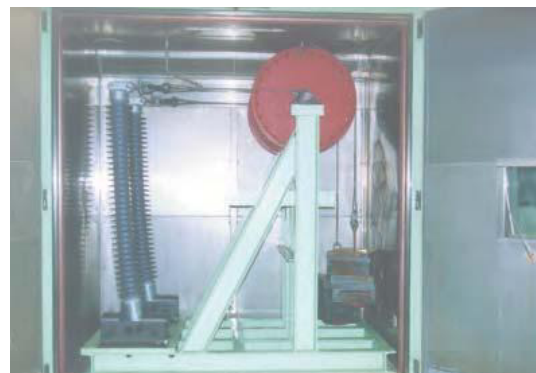
Cantilever Load Test Facility in Thermal Cycle Chamber
