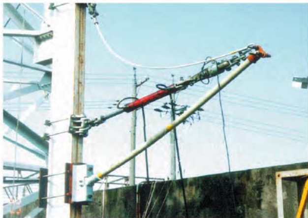
Fig. 6 - One axis testing (transverse compression load)
